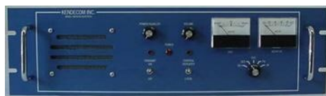
ACARTS 146.88(-) W9INX Kendecom KRP5000 VHF Analog Repeater (Soon to be tested on 146.880)
